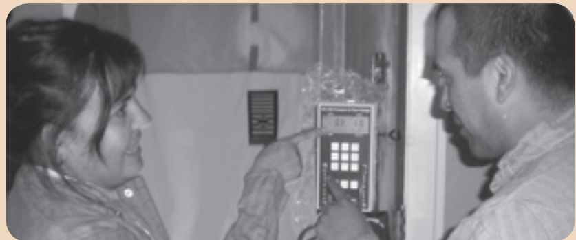
Berenice Lopez-Dorsey working with employee Javier Hilario running a Blower Door to test the air leakage in a Portland-area home.
